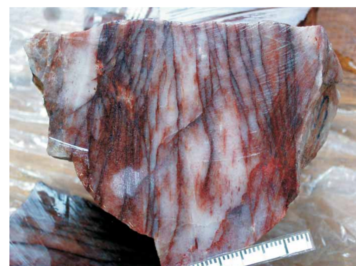
Fig 22. Slab with series of closely-packed, subparallel sheeted veinlets filled by magnetite and sulfides hosted in a quartz pod. Oxidation of the sulfides produced goethite coloration in parts of the sample. Comes from part of an IOCG mineralised system. Again, quartz pods are hosting mineralisation. Each black or white mark in scale is 1 mm.
