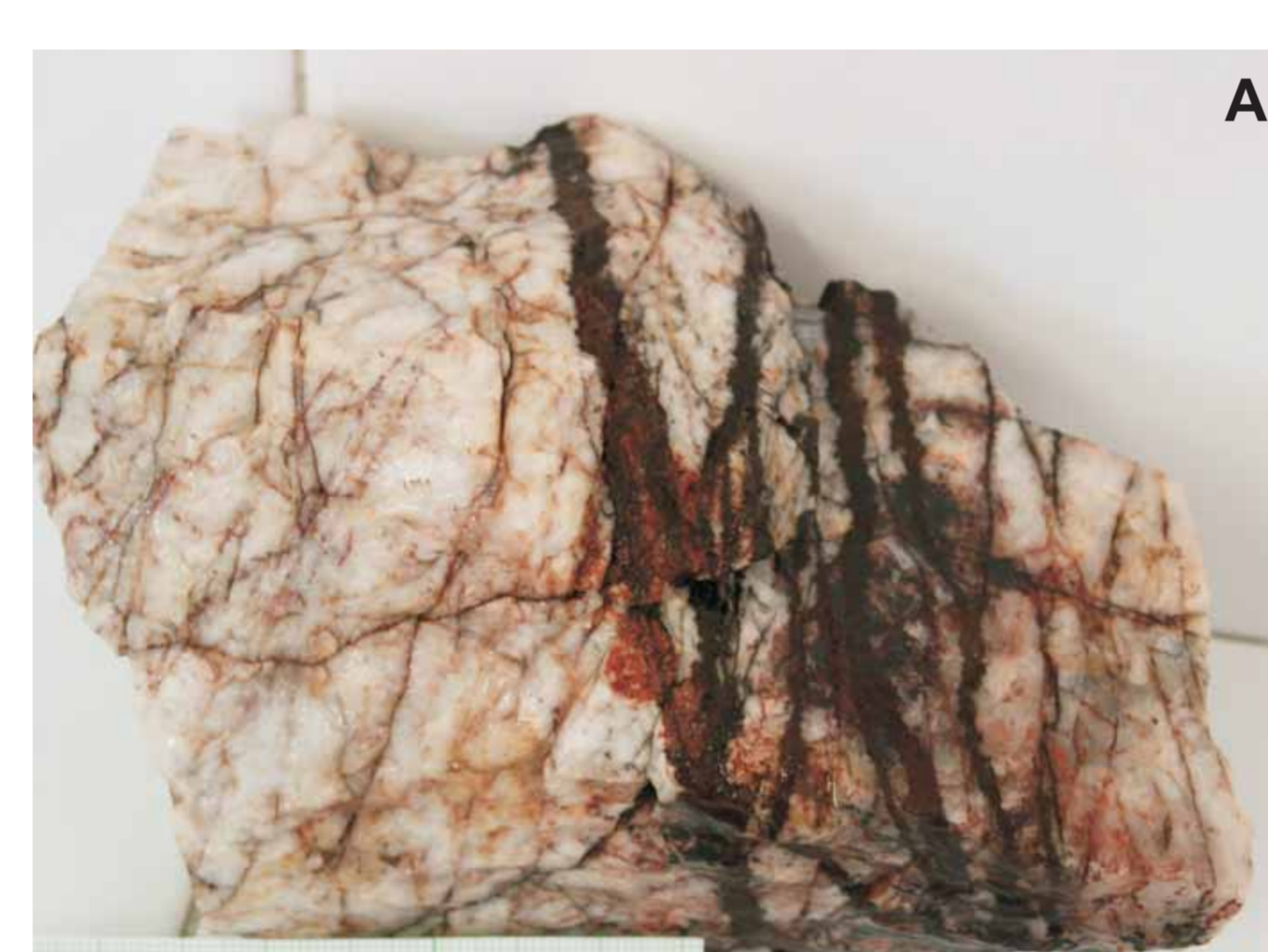
Fig 18. Slab of a copper sulfide-rich, magnetite stockwork hosted in a quartz pod. The field of view is 15 cm. Note copper carbonates after bornite and chalcopyrite. Brown-red stains are hematite, after pyrite mineralization in the veinlets. These features are common in portions of some quartz pods, and may extend for several dozens of square meters in outcrops.
