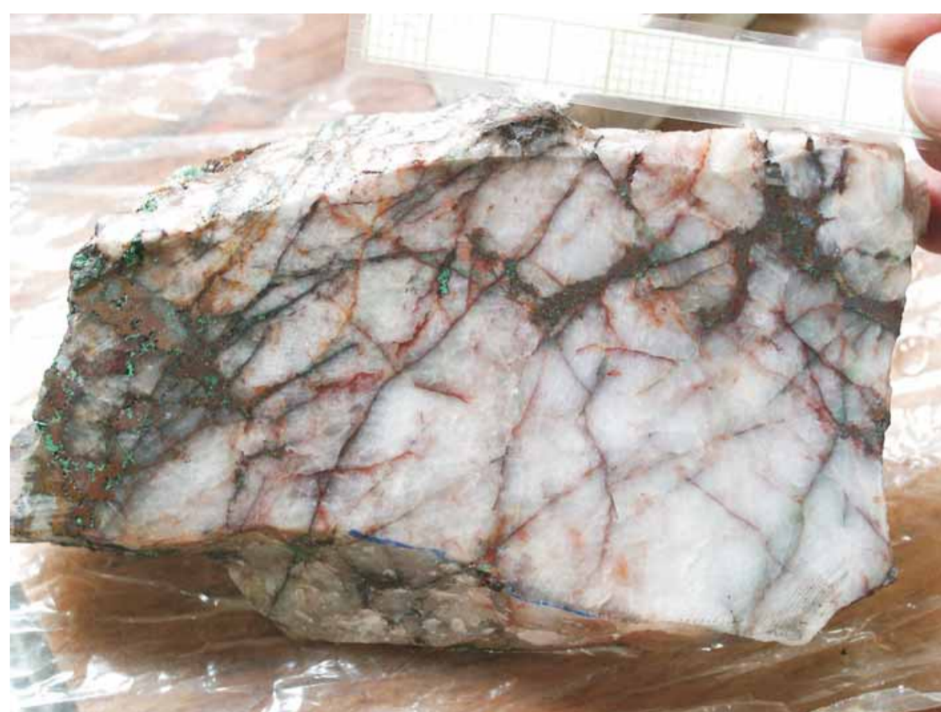
Fig 18. Slab of a copper sulfide-rich, magnetite stockwork hosted in a quartz pod. The field of view is 15 cm. Note copper carbonates after bornite and chalcopyrite. Brown-red stains are hematite, after pyrite mineralization in the veinlets. These features are common in portions of some quartz pods, and may extend for several dozens of square meters in outcrops.
