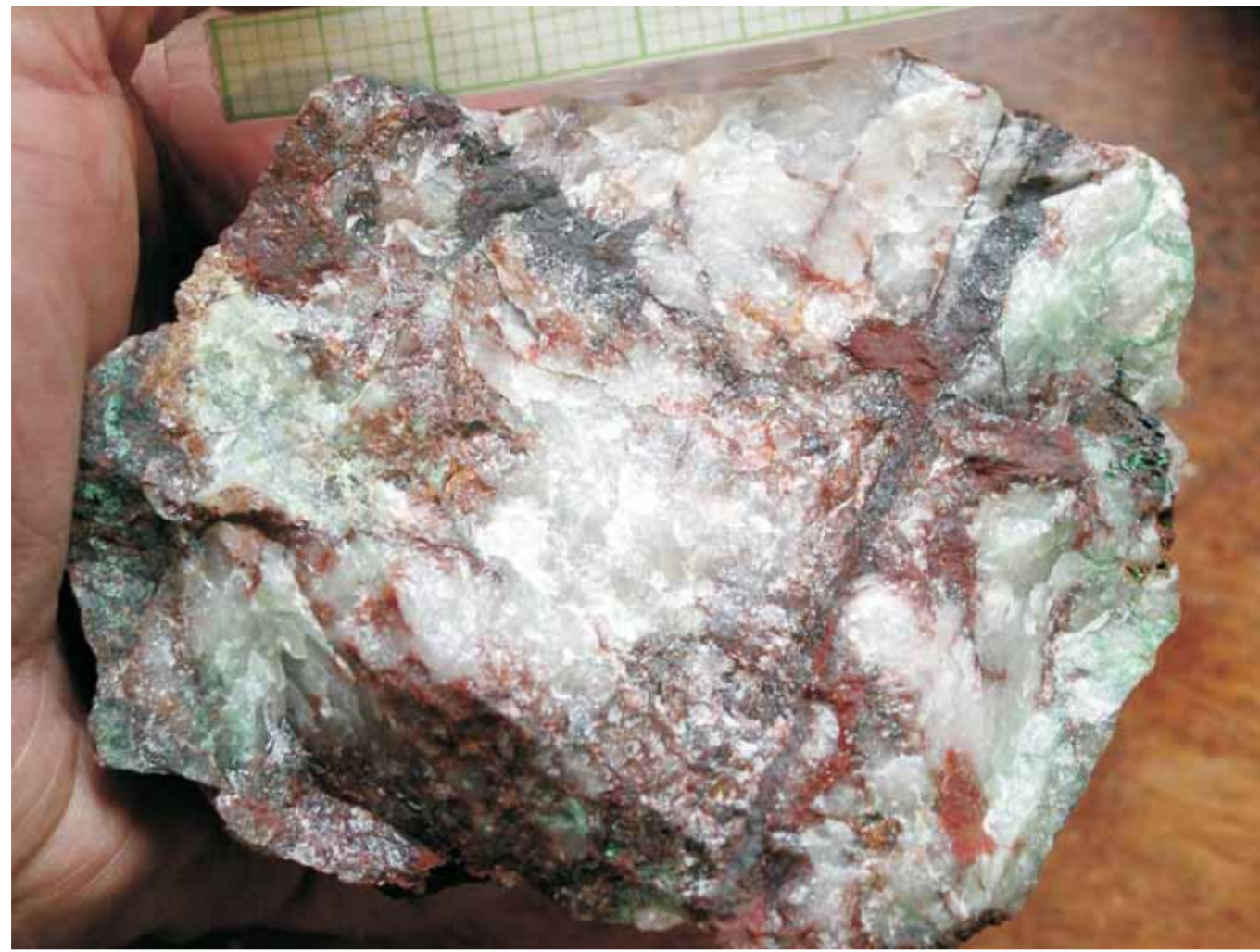
Fig 16. Portion of a chalcopyrite-pyrite rich, magnetite-filled stockwork in a quartz pod. Note some of the vugs. Scale has marks every 2 mm.
