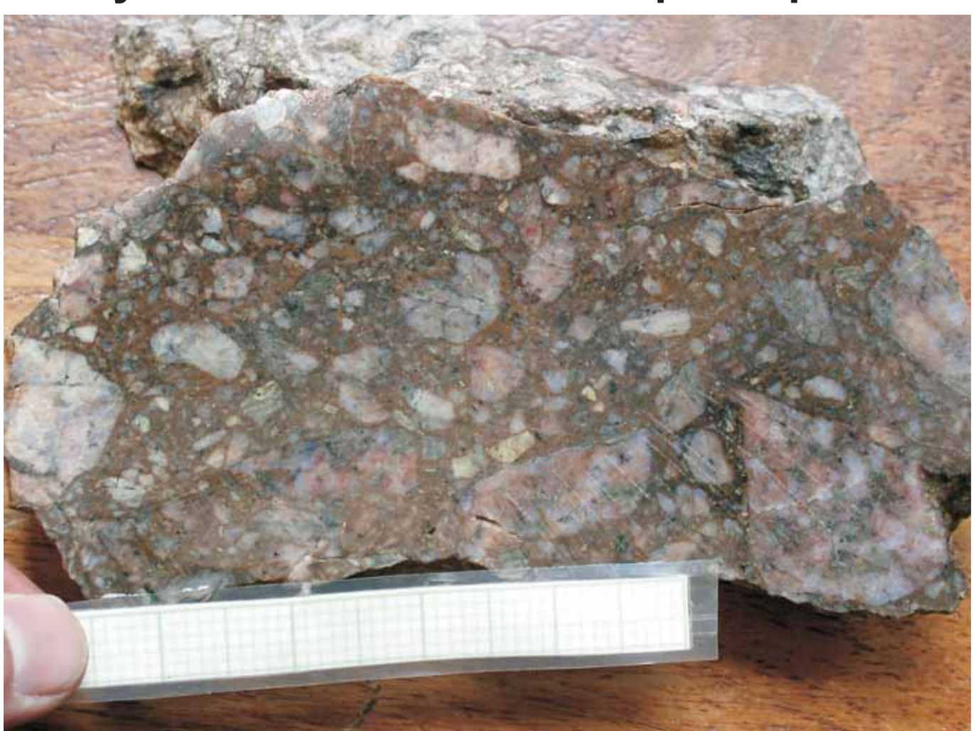
Fig 19. Monomict, explosive hydrothermal breccia from the Teverede rich Cu+Au IOCG project, northwestern Kamanjab Batholith, Namibia. Fragments are rounded to sub-angular. Quartz pods are both host rocks and single clast component for this breccia. Quartz pods behave in a brittle way and produce very important brecciation around IOCG systems. Scale with marks every 2 mm.
