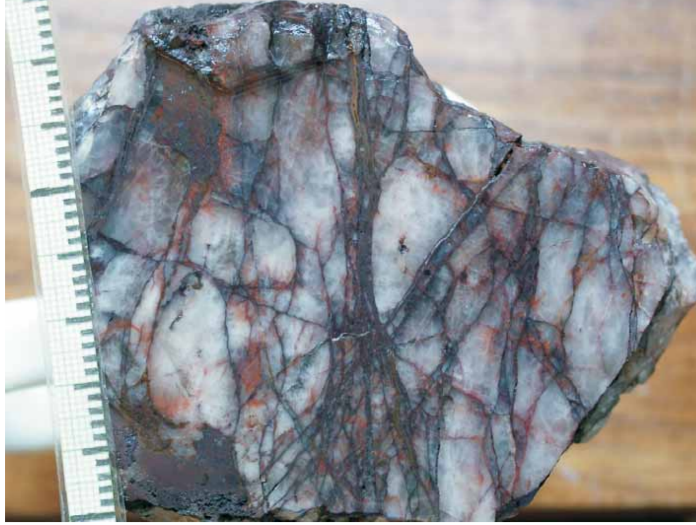
Fig 15. Dense network of magnetite-pyrite-chalcopyrite veinlets in a quartz pod. This particular outcrop has at least 150 m in diameter, and contains significant copper mineralization. Gold might also be present in economic concentrations. Scale marks every mm.
