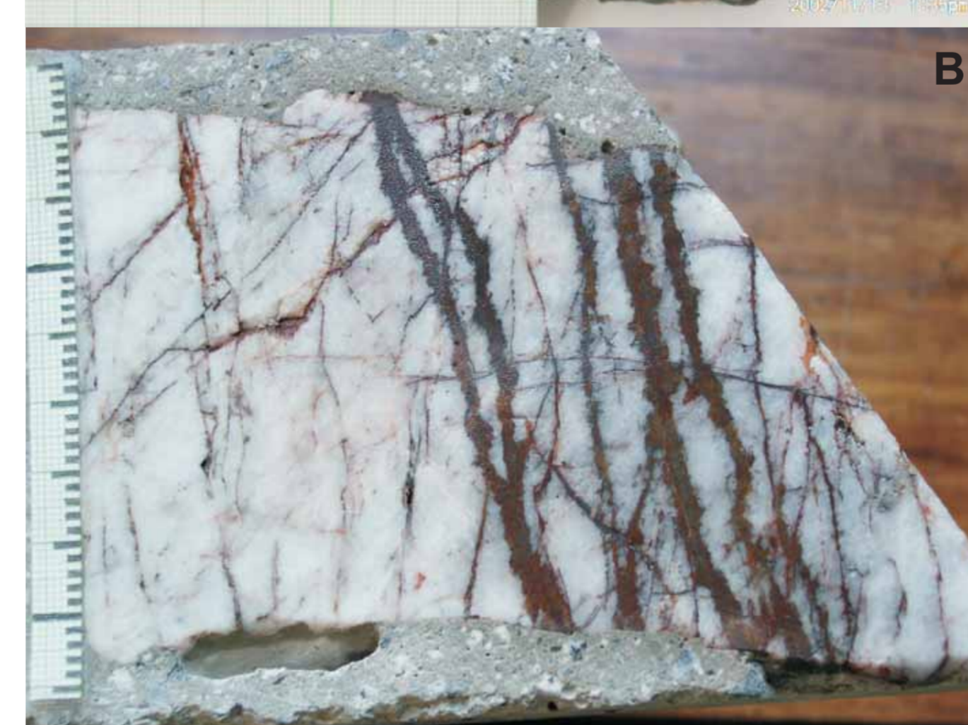
Fig 21. Braided veins with hematite and oxidized sulfides that are hosted in a quartz pod. The sample was very fragile and was set in concrete for slabbing. Notice several generations of fractures that intersect each other. If mineralized with gold, such a sample could carry milligrams per ton. Outcrop surface above, slabbed surface below. Collected at the Oas farm, Khorixas inlier, Namibia. Both scales in mm.
