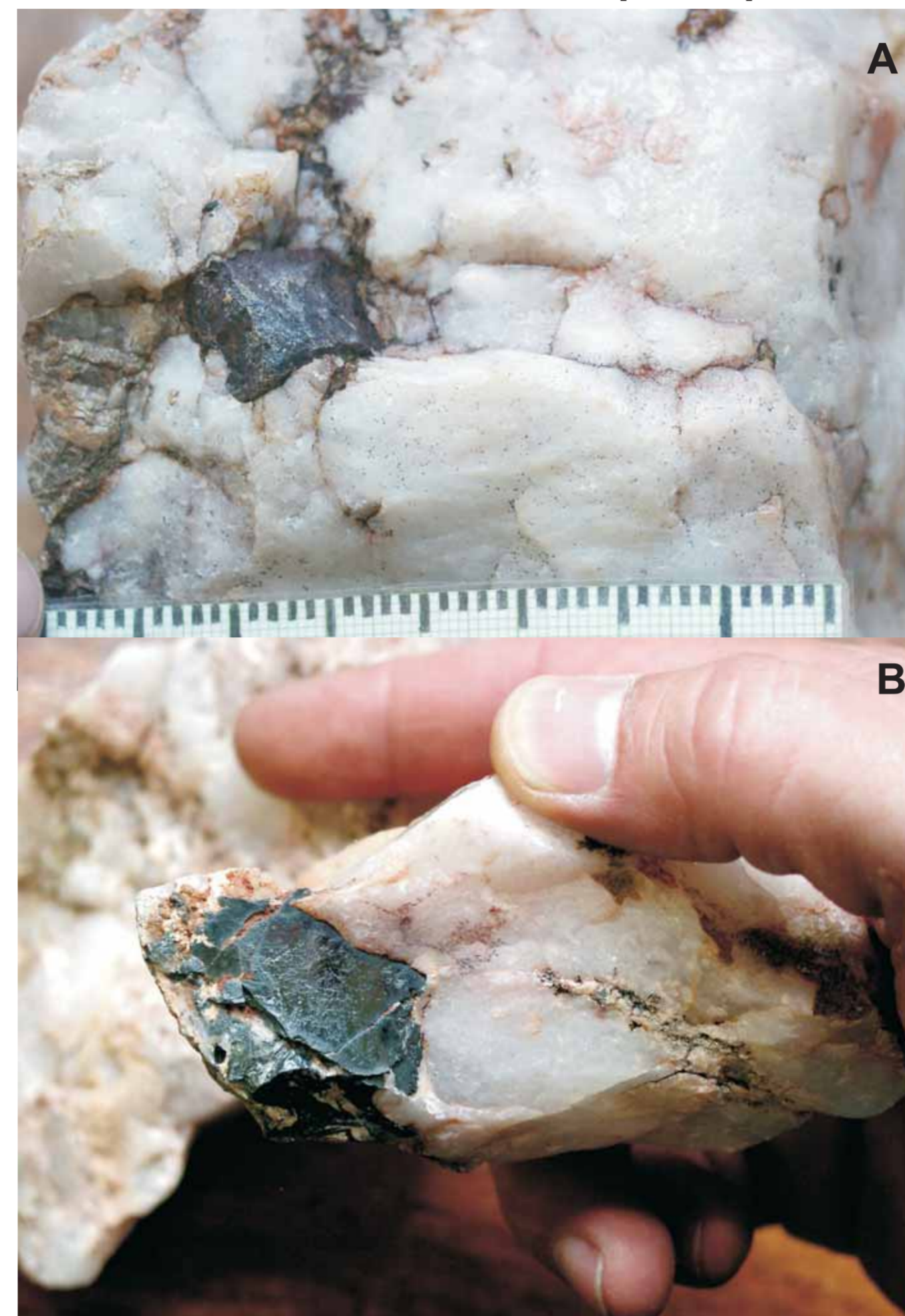
Fig 8. Isolated, cubic magnetite crystals hosted by quartz pods. Scale marks every millimeter.
