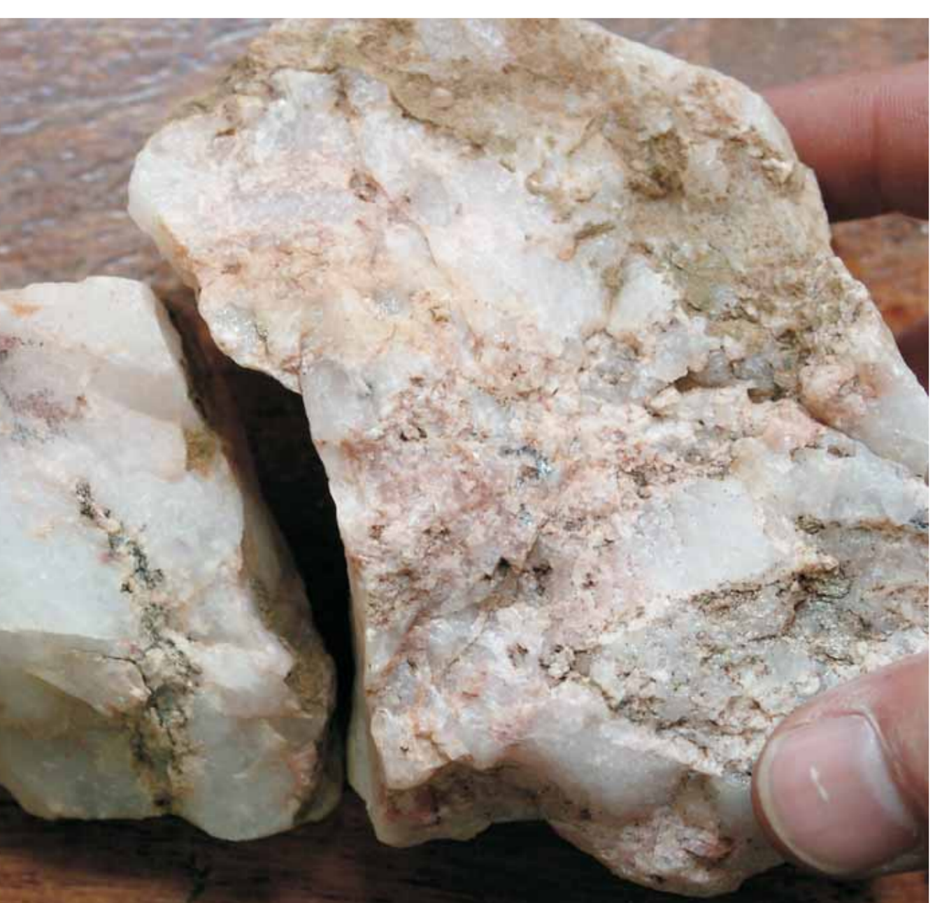
Fig 4. Close-up view of a fragment from a quartz pod. Pink color is due to small particles of hematite in the quartz. The sample was taken from a round outcrop, 80 meters in diameter. The thumb is 2.2 cm wide.
