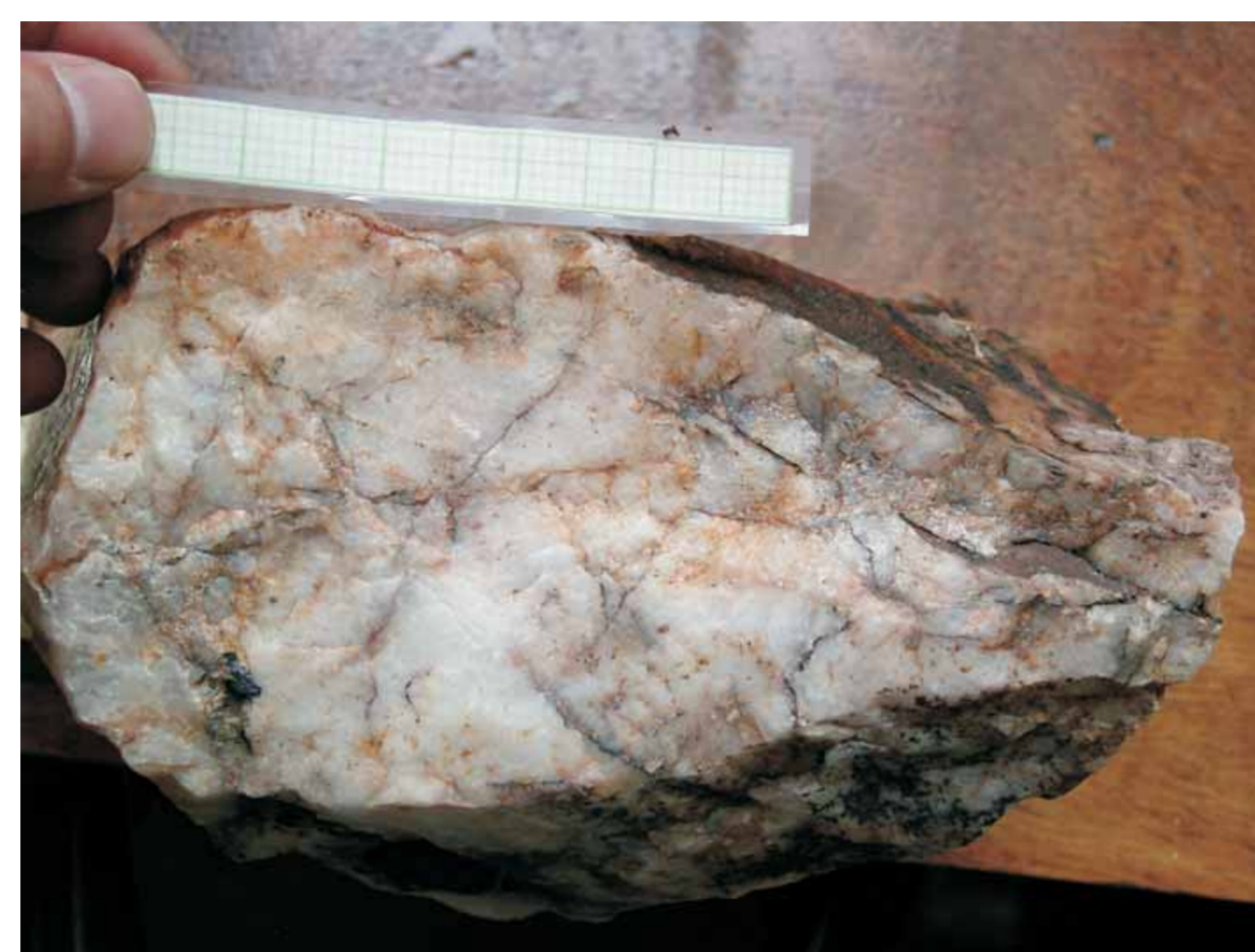
Fig 5. Massive quartz from a quartz pod. It shows minor iron oxide veinlets. This is the way most quartz pods are seen on outcrops. Marks every 2mm.
