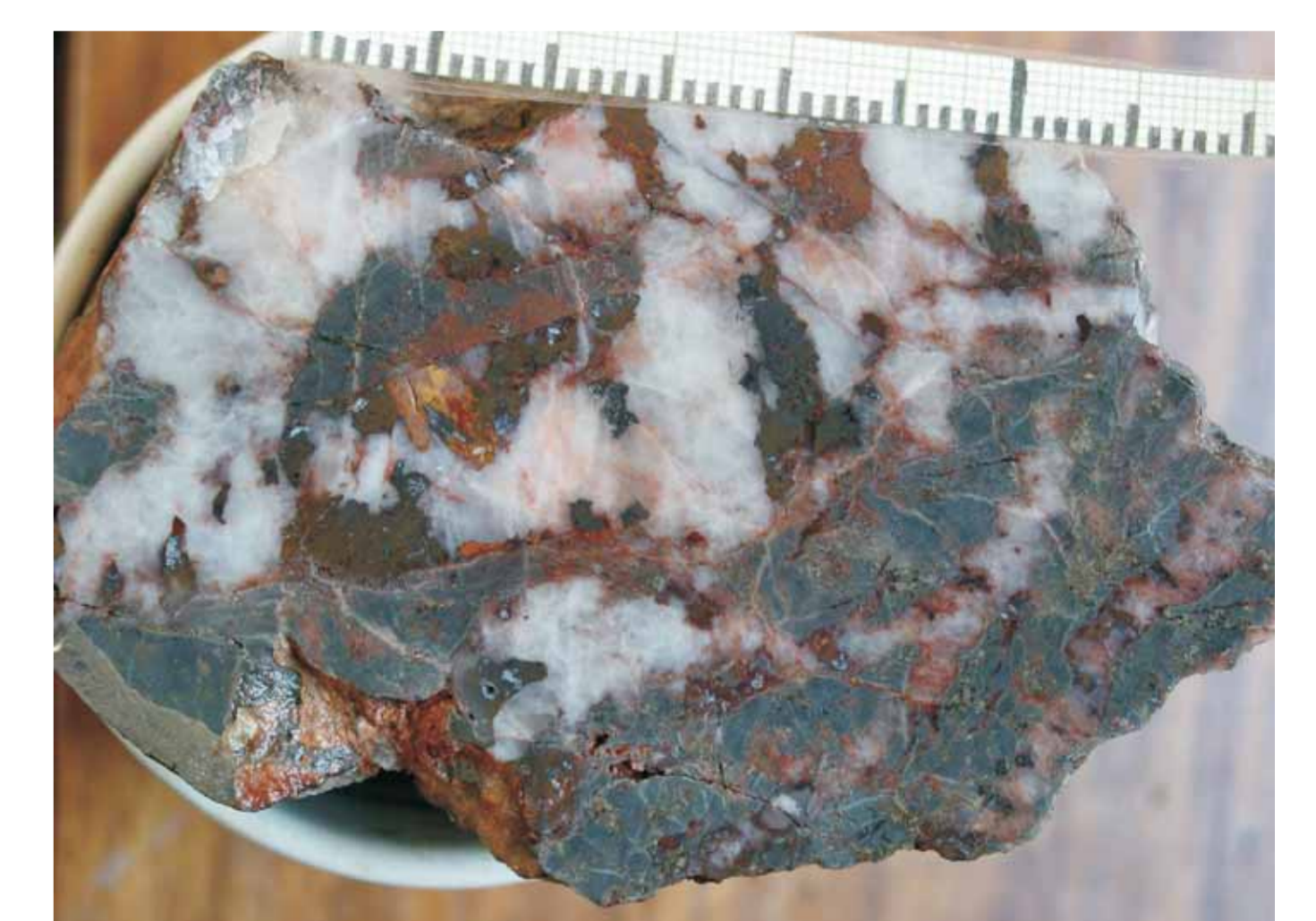
Fig 14. Slab of a densely-mineralised quartz pod. Massive hematite with minor pyrite progressively overprint quartz to leave very little of the original quartz. Scale in mm.
