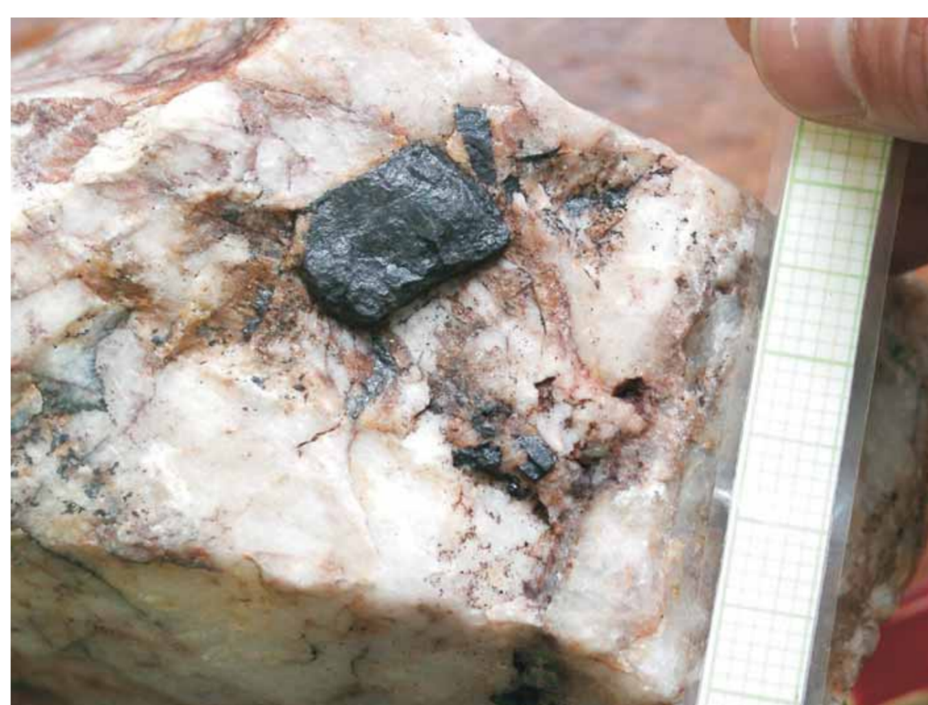
Fig 10. Sub-rounded magnetite crystal found inside a quartz pod. This is an uncommon feature. The largest crystals observed are 8 cm in diameter and were found in the Egue site, NE of Otjiwarongo, Namibia (Fig 26). The origin of these iron oxide crystals is not well understood. Magnetite phenocrystals seem to have formed in a space that allowed free ion migration, possibly in gel state, but definitely before the quartz was solid. Maybe the quartz flowed and euhedral magnetite crystals were transported along. Scale marks every 2 mm.
