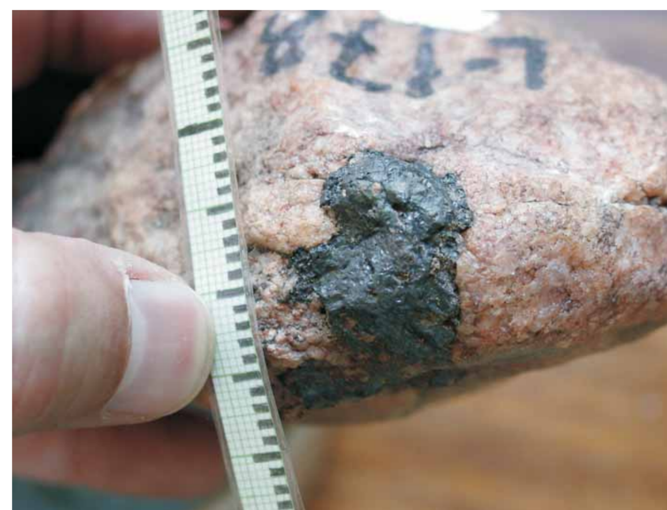
Fig 9. Corroded hematite-martite crystal hosted in a quartz pod. This type of inclusion is not common. The hematite crystal is not euhedral as in other cases (Fig 8), but displays irregular rims. Scale in mm.
